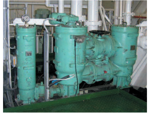
2-Stroke Diesel Marine Engine MAN B&W 6S35MC Ship "TRANS EMERALD" DACX-RM Filter Filtration 40 µm
